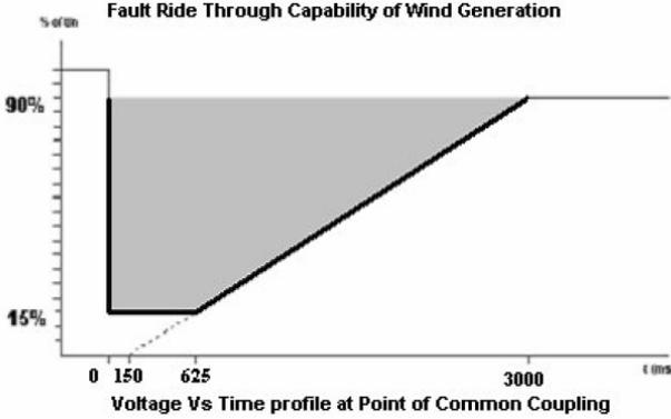
Fig. 1. E.ON Netz voltage dip curve.
