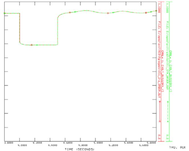
Fig. 12. Voltage at Bus 6 (220 kV). Red solid line: third order model. Green dashed line: fifth order model.
