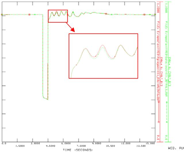
Fig. 14. Voltage at Bus 1 (132kV). Red solid line: equivalent model. Green dashed line: detailed model.
