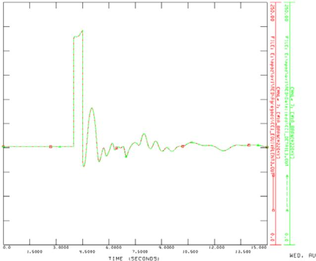
Fig. 17. MVA flow at Line 2. Red solid line: equivalent model. Green dashed line: detailed model.
