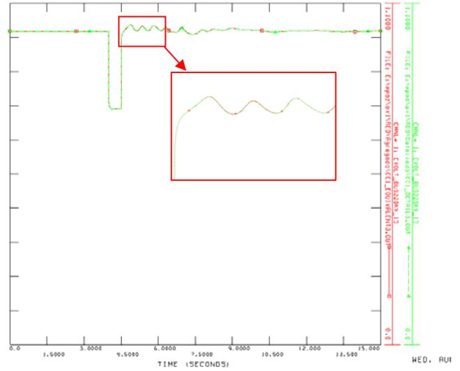
Fig. 15. Voltage at Bus 6 (220 kV). Red solid line: equivalent model. Green dashed line: detailed model.
