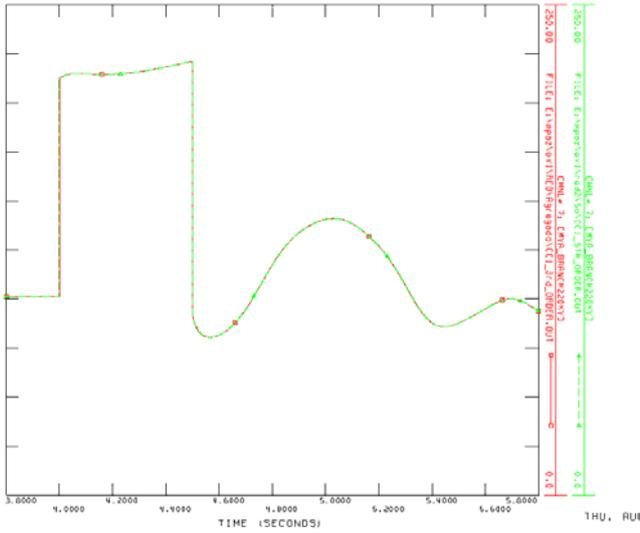
Fig. 13. MVA flow in Line 2. Red solid line: third order model. Green dashed line: fifth order model..
