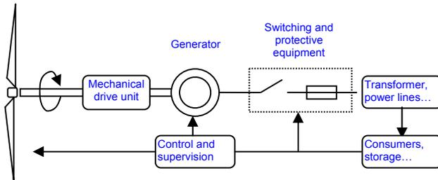
Fig. 2. Fixed speed wind turbine scheme.
