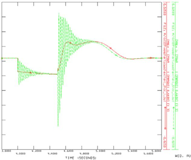
Fig. 10. Wind turbine generated power. Red solid line: third order model. Green dashed line: fifth order model.
