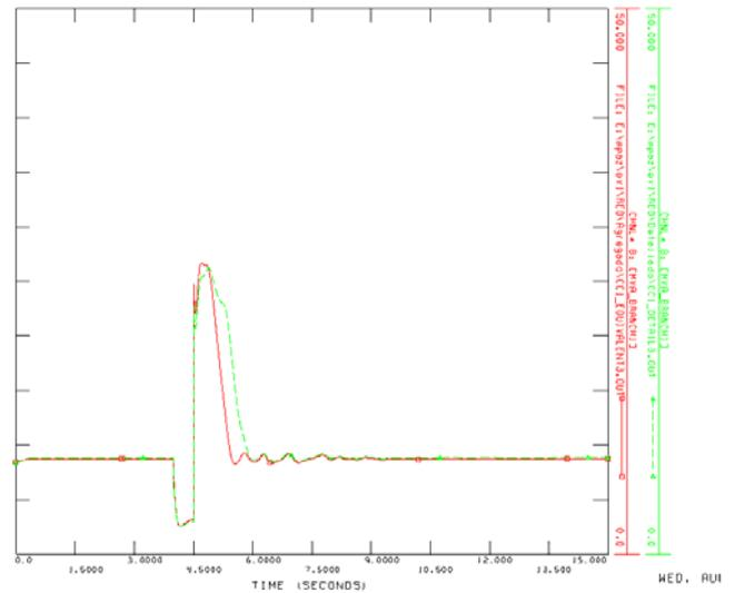
Fig. 16. MVA flow at Line 1. Red solid line: equivalent model. Green dashed line: detailed model.
