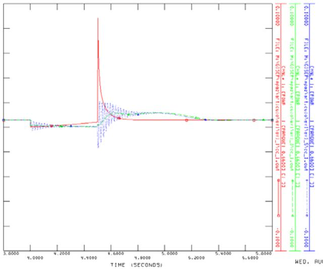
Fig. 9. Wind turbine generated power. Red solid line: first order model. Green dashed line: third order model. Blue dotted line: fifth order model.
