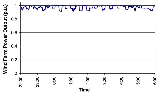
Fig. 3: Active power output of a wind farm with 26 turbines experiencing repetitive connection and disconnection of up to two turbines due to internal errors in 7/02/1999 (mean speed at meteorological mast was around 14 m/s).
