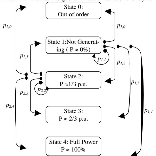
Fig. 9: Discretization of power output of one wind farm into a number of states (four in this figure). Only transitions from states 1 and 2 are shown for clarity.
