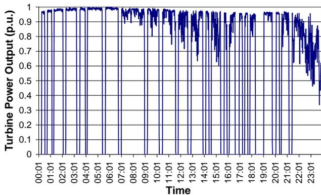
Fig. 2: Power output of a single turbine experiencing 24 repetitive stops due to over temperature in 20/07/1998 (24 h).
