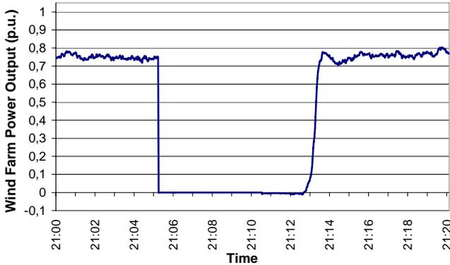
Fig. 6: Active power output of a wind farm experiencing a disconnection in 3/02/1999 due to a trip of the homopolar protection relay between 21:05:24 and 21:10:55. Three minutes later, the output reached normal values.
