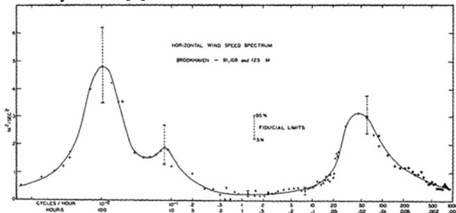
Fig. 1: Van der Hoven's spectral model (from [1]).
