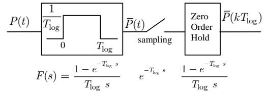
Fig. 7: Model of the wattmeter of the wind farm.
