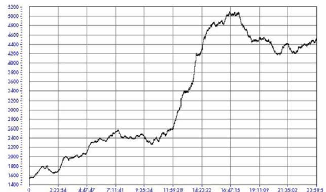
Fig. 5: Active power output (MW) of Spanish wind farms experiencing high increase in 18/01/2005 between 12:00 and 15:00.
