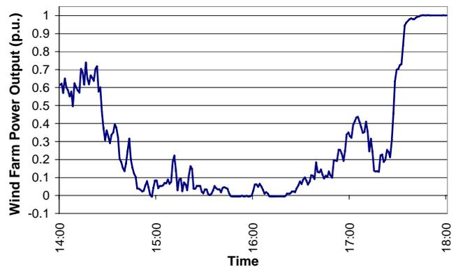
Fig. 4: Active power output of a wind farm experiencing high variability in 9/02/1999 due to a sudden change in the weather at 17:30.
