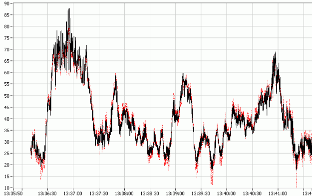
Fig. 207: Rective power Q [kVar] (in solid black line) of a SCIG 600 kW wind turbine for series #1, corresponding to Fig. 200, and its linear estimation from real power.
