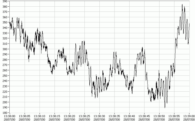
Fig. 202: Detail of real power of a SCIG 600 kW wind turbine for wind speeds around 9,5 m/s during 1 minute in series #1.
