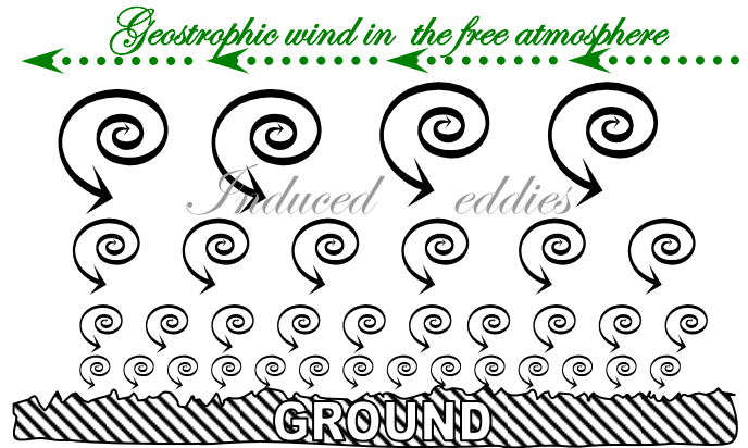
Fig. 3: Schematic of eddies as a function of height at atmospheric boundary layer. Taken from Simon Watson [56].
