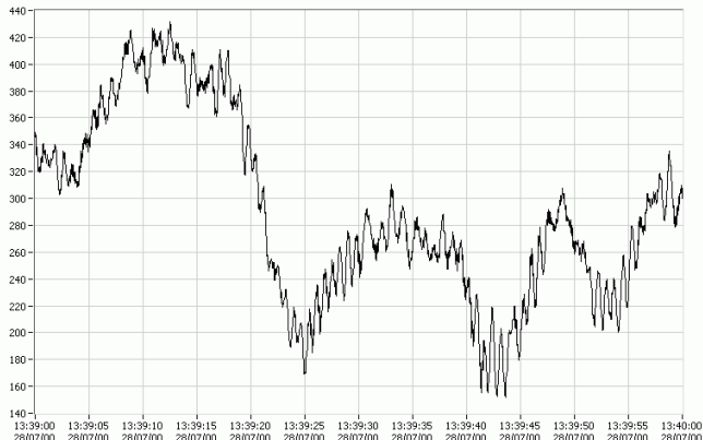
Fig. 203: Detail of real power of a SCIG 600 kW wind turbine for wind speeds around 7 m/s during one minute in series #1.
