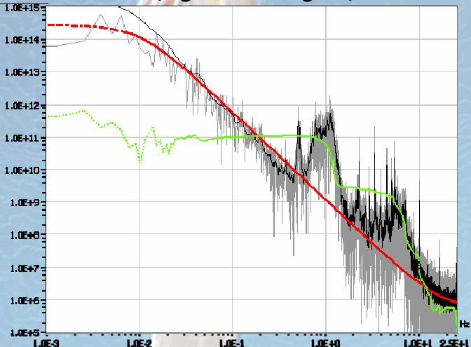
Fig. 2: PSD of active power of a fixed speed, stall regulated turbine at low winds (parameterization in red, accumulated error of the parameterization in green).
