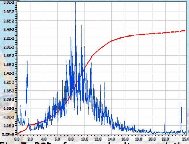
Fig. 7: PSD of squared voltage variations  $b(t)$  and  $\sigma_b^2|_{f_{\max}}$  in a doubly fed induction generator.
