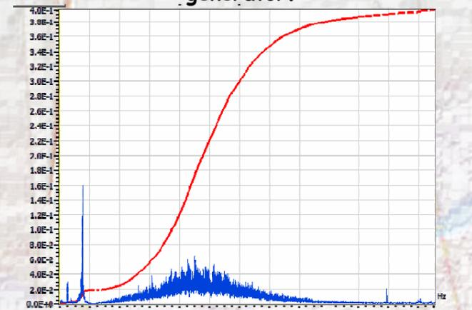
Fig. 8: PSD of squared voltage variations  $b(t)$  and  $\sigma_b^2|_{f_{max}}$  at a wind farm with 17 doubly fed induction generators.
