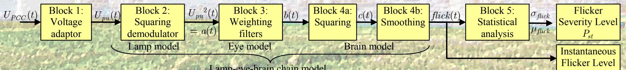
Fig. 1: Simplified block diagram of IEC Flickermeter according to IEC 61000-4-15
