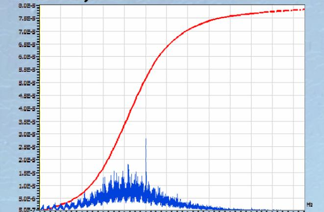
Fig. 6: PSD of squared voltage variations  $b(t)$  and  $\sigma_b^2|_{f_{max}}$  in a variable resistance induction generator (opti-slip) wind turbine.
