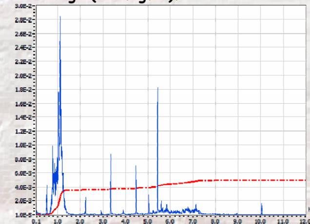
Fig. 5: PSD of squared voltage variations  $b(t)$  and  $\sigma_b^2|_{f_{max}}$  in a fixed speed, stall regulated wind turbine (contribution of each frequency in blue, accumulated flicker contribution in red).
