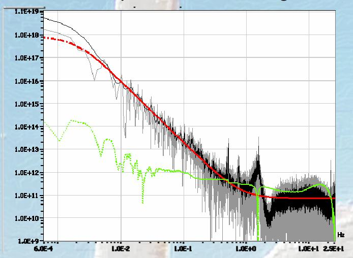
Fig. 3: PSD of a doubly fed, induction generator wind farm at low winds.
