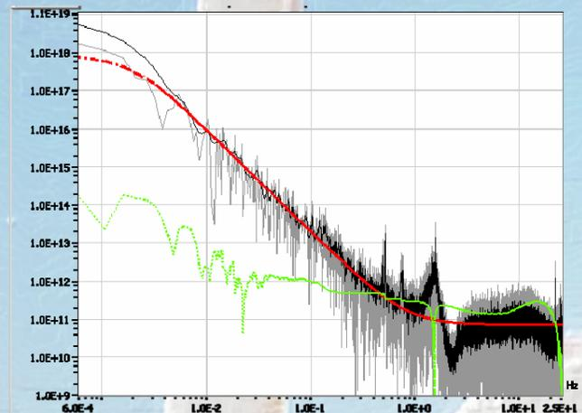
Fig. 3: PSD of a doubly fed, induction generator wind farm at low winds.
