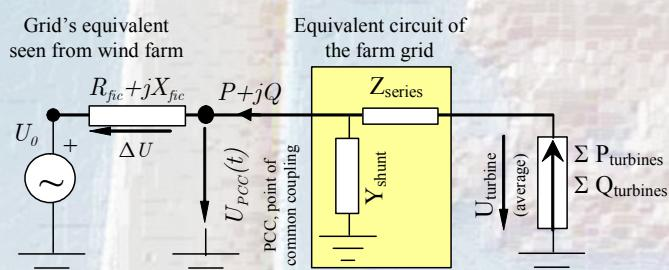
Fig. 4: Small signal model of the farm.
