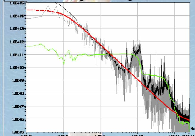
Fig. 2: PSD of active power of a fixed speed, stall regulated turbine at low winds (parameterization in red, accumulated error of the parameterization in green).
