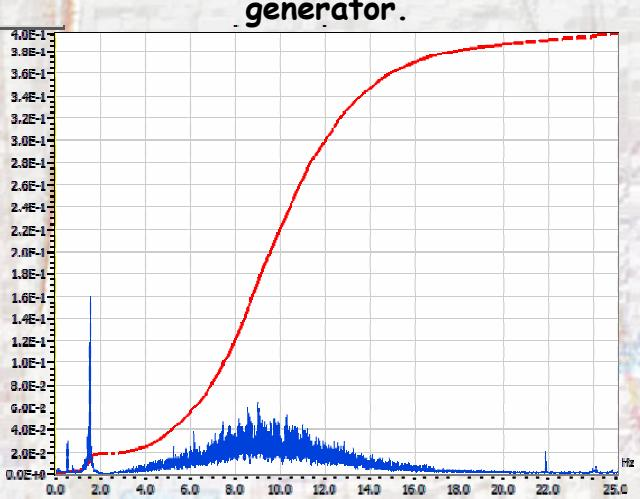
Fig. 8: PSD of squared voltage variations  $b(t)$  and  $\sigma_b^2|_{f_{\max}}$  at a wind farm with 17 doubly fed induction generators.
