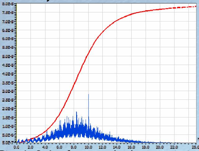
Fig. 6: PSD of squared voltage variations  $b(t)$  and  $\sigma_b^2|_{f_{\max}}$  in a variable resistance induction generator (opti-slip) wind turbine.
