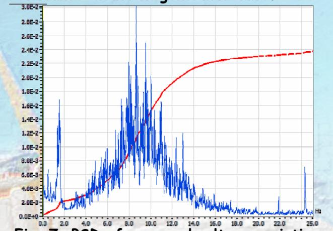
Fig. 7: PSD of squared voltage variations  $b(t)$  and  $\sigma_b^2|_{f_{max}}$  in a doubly fed induction generator.
