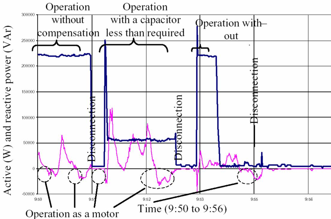
Fig. 2: Active and reactive power of a VRIG WT along the time (1 min averages).
