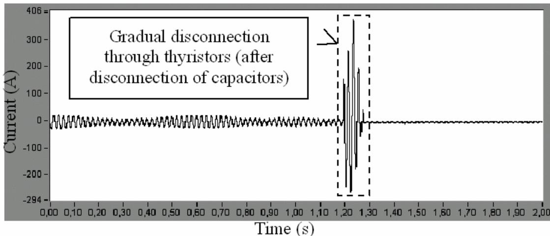
Fig. 4: Current waveform at VRIG during a disconnection.
