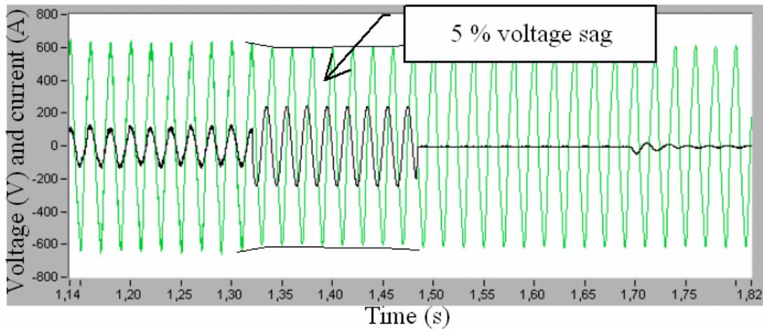
Fig. 5: Current (black) and voltage (grey/green) waveforms at DFIG during a disconnection.
