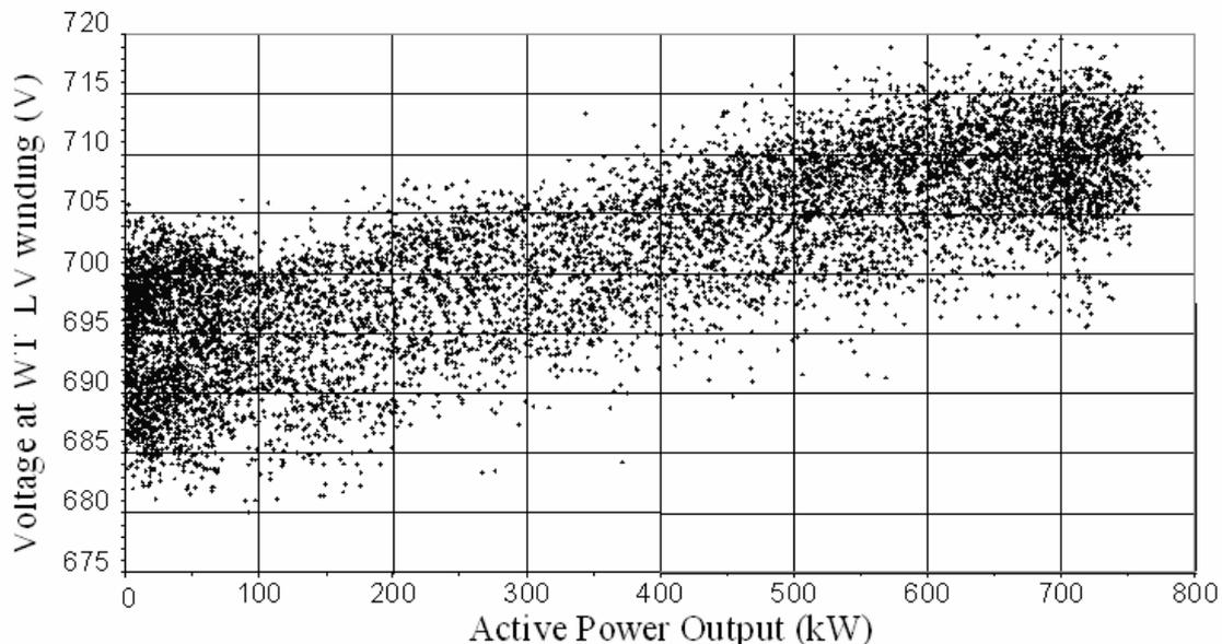
Fig. 2: Voltage versus power output at a SQIG WT connected to a quite resistive line.
