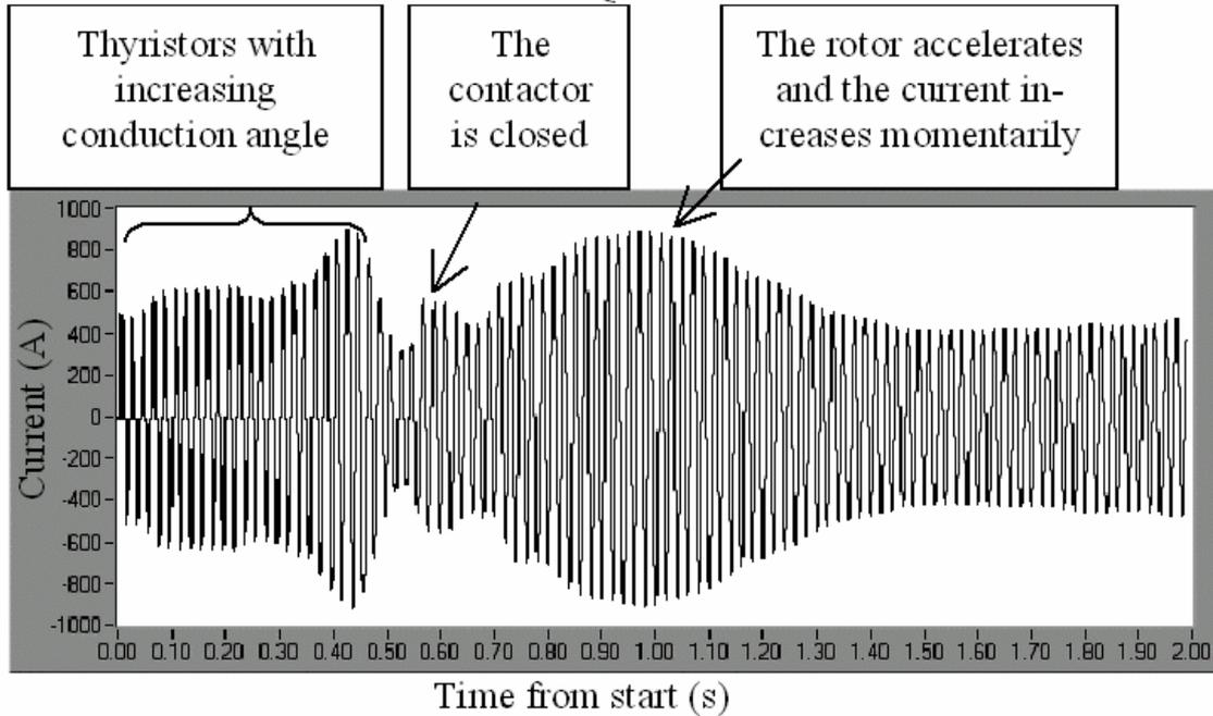
Fig. 3: Intensity of current during the connection of SQIG.
