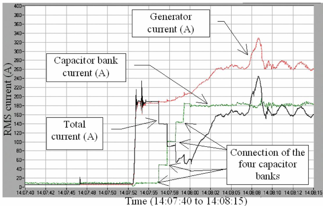
Fig. 6: Phase-to-neutral voltage, current and power during the connection of VRIG.
